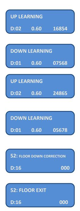
If you see this message on the screen, in 1. Up learning, the elevator goes at high speed, slows down to a lower floor of the top floor, goes to the top floor at approaching speed and stops when it sees the ML, ML2 magnet.
